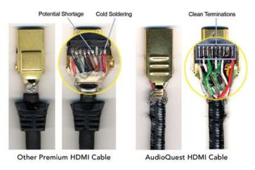
Soldering versus crimping connection.
