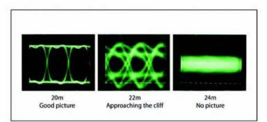
*Eye Pattern test shows the waveforms of the digital signal (bits) visually. It also shows the Cliff Effect.*
