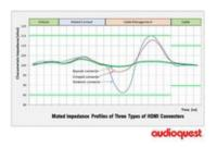
Click on image to see TDR results of AudioQuest's Bayonet connector versus traditional soldered and crimped connectors. AudioQuest's single-conductor design gives the company an advantage when it comes to field termination.
