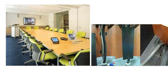
In Presenter conference rooms, you only need to run one Cat6 cable between Tx boxes, and one Cat6 cable to the projector; the Show Me button can replace the control system; VGA, HDMI and DP are all working together and the system is scalable
