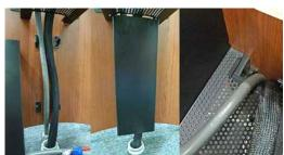
In Presenter systems, there's only one Cat6 cable at any point of the system (in and out from the yellow connectors); no more centralized switchers!
