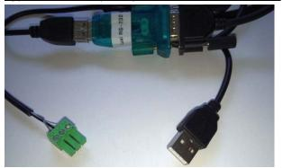
The USB connector is most commonly seen on laptop computers. There's an electronics circuit board in between and comes with a USB driver for that circuit. Please load the driver to the laptop first. Regardless what connector is on the opposite side, follow the instructions above to cut off, strip and screw on the 3 wires to the provided 3-pin captive screw plug.
