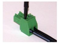
same location, one Luxi external power supply can power up to 5 units. Use extra insulated wires (18 AWG to 22 AWG) daisy-chain the multiple power input captive screw plugs, connecting all positive side together, and connecting all negative side together.
