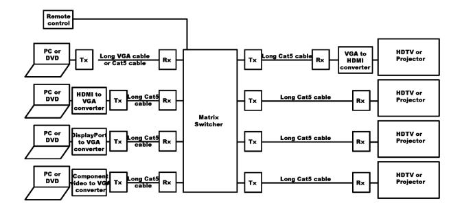
These kinds of systems work well, especially for the small system with few I/Os (inputs and outputs). Without the alternatives, we have accepted this as the de facto standard even it has several major challenges:
