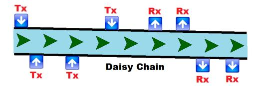
Multiple signals are allowed to flow thru the daisy chain (river) to achieve true matrix switching. See the system diagrams below:
