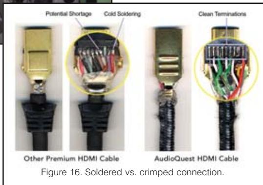
Figure 16. Soldered vs. crimped connection.
