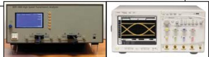
Figure 12. BER and Eye Pattern test equipment.
