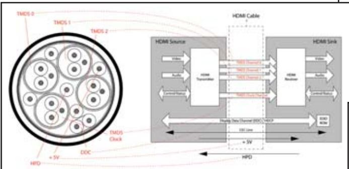
Figure 1. Components inside an HDMI cable. All the signals travel inside one HDMI cable.
