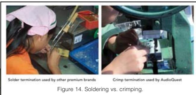
Figure 14. Soldering vs. crimping.
