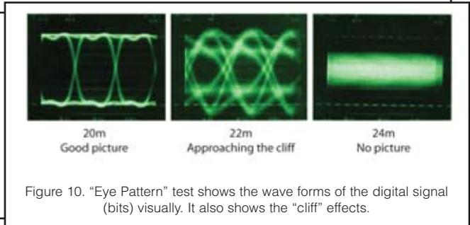
Figure 10. “Eye Pattern” test shows the wave forms of the digital signal (bits) visually. It also shows the “cliff” effects.
