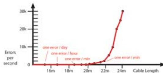
Figure 11. BER test also shows the “cliff” effects.
