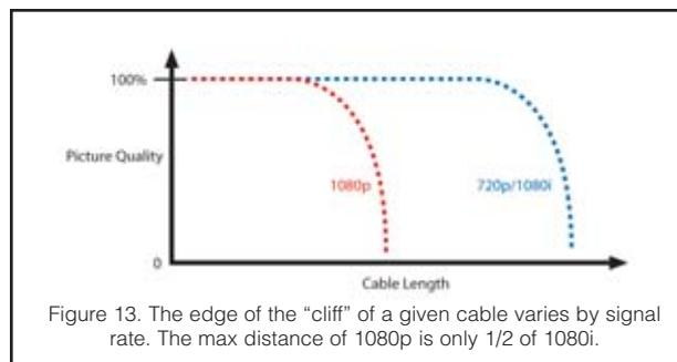
Figure 13. The edge of the “cliff” of a given cable varies by signal rate. The max distance of 1080p is only 1/2 of 1080i.
