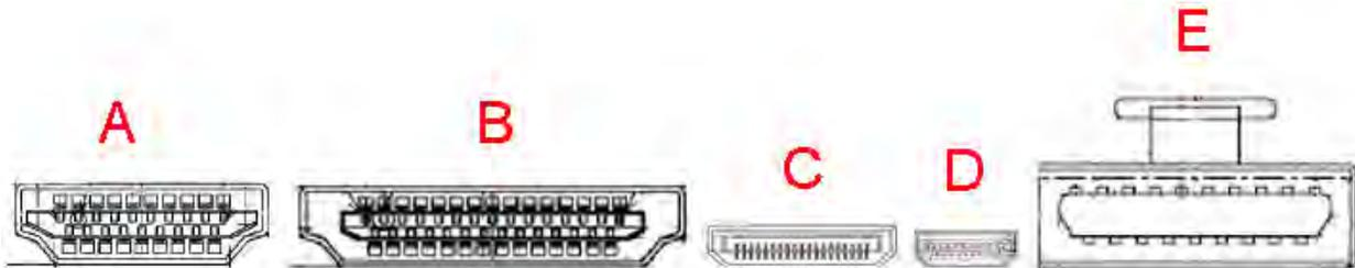
Fig. 5 HDMI plug types
