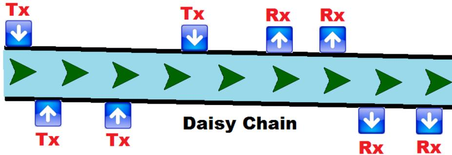
Multiple signals are allowed to flow thru the daisy chain (river) to achieve true matrix switching. See the system diagrams below:
