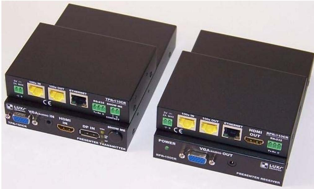
The 2 smaller boxes on top are the simplified Tx and Rx without scaler; the 2 bigger ones on the bottom are the Tx and Rx with built in scalers. The highly visible yellow RJ45 connectors are for daisy chain input and output.
