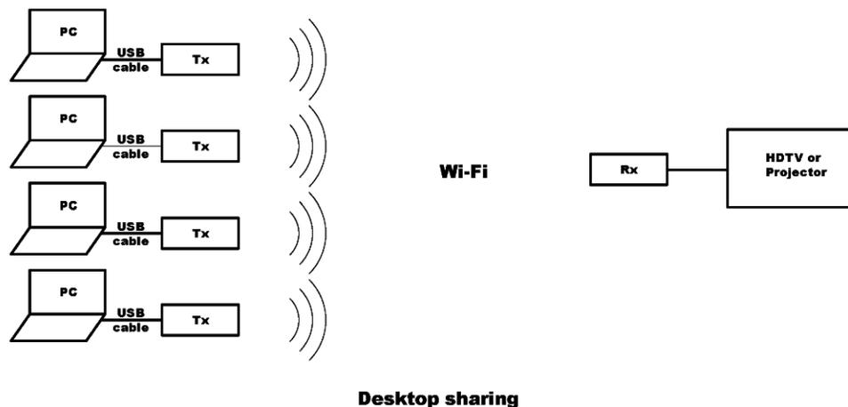
A small box connects to each PC via a USB pigtail. The software takes a snapshot of the PC desktop screen, and sends it to the receiver via Wi-Fi. Each box also has a click button on top. If one button is clicked, the desktop of the connected PC would be sent to the receiver and displayed on the projector. If more than one button is clicked, the desktop screenshots of the associated PCs would be shown on the projector as small windows.
